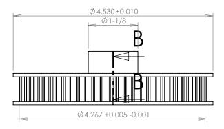
**NOTE: CORED PULLEYS** HAVE 1/16" THICK RIBS, REINFORCEMENT
